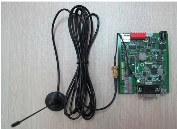
Figure 1. The IEEE802.15.4c-based communicator
