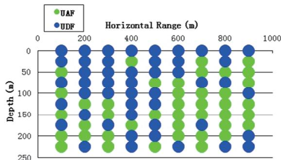
Fig. 8: Hybrid Forwarding Scheme with Minimum BER
