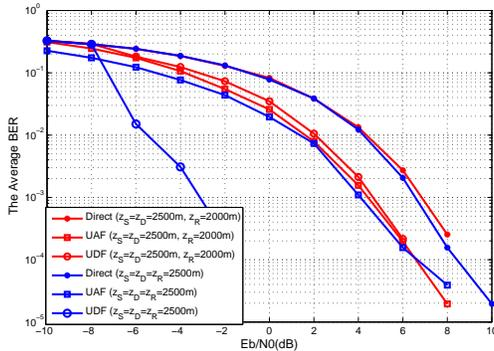
Fig. 5: BER Performance with Varying SNR of the S to D link for Two Topology Deployments
