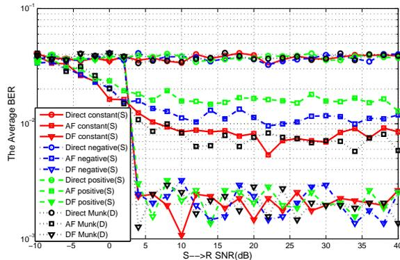
Fig. 4: BER Performance for UAF, UDF and Direct Transmission, under Different Underwater Channels.
