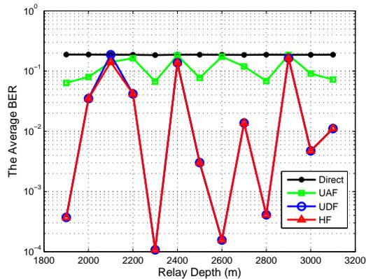
Fig. 7: BER vs. Relay Depths
