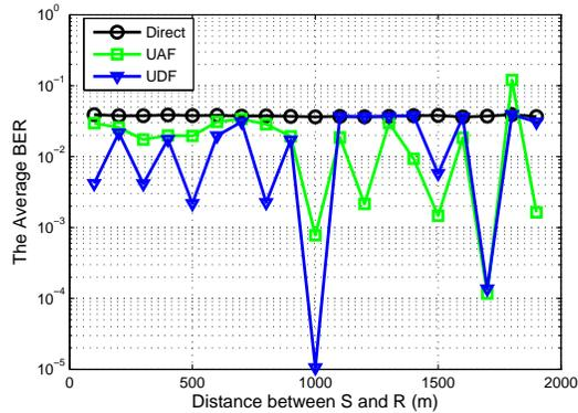
Fig. 6: BER vs. SR ranges, Near the Sea Bottom
