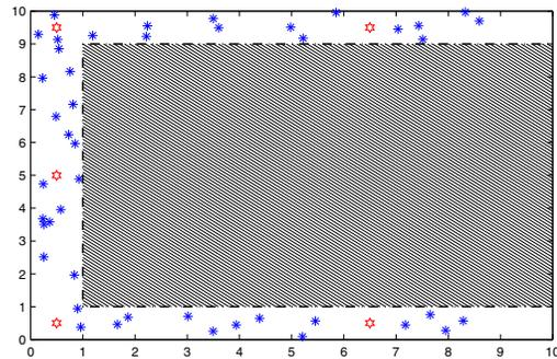
Fig. 2. Example of C-Shape Topology with 50 nodes randomly deployed, red stars are anchors, blue asterisks are unknown nodes
