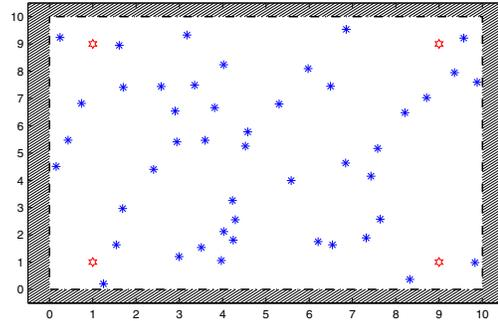
Fig. 1. Example of Square Topology with 50 nodes randomly deployed, red stars are anchors, blue asterisks are unknown nodes
