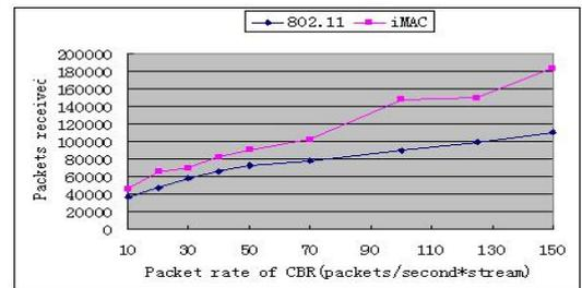
Figure 4.2 Throughput (velocity: 10m/s)
