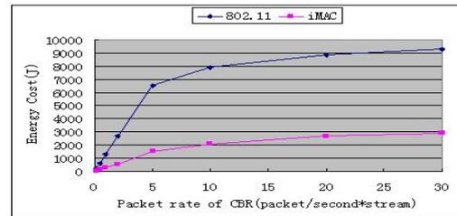
Figure 4.6 Energy Consumption (static topology)
